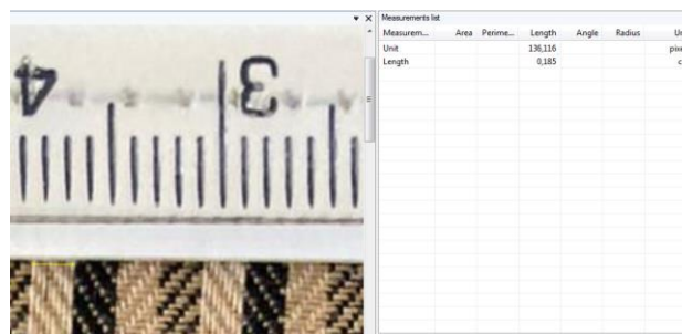
Figure 3. Measuring the yarn density per area
